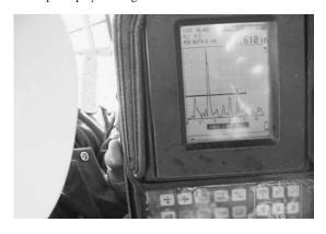
these errors should be made with a flaw detector. A flaw detector provides better penetration, more efficient scanning, high temperature measurement capabilities, flexibility with a variety of transducers and better screen update capability.
