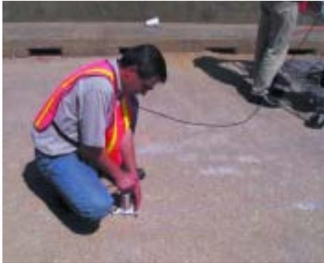
Figure 3. Impact echo is useful in determining slab thickness, voids and subsurface discontinuities. Concrete surface is impacted with hardened-steel ball to generate stress waves.
