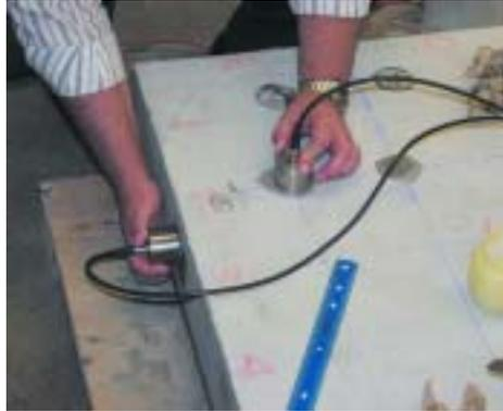
Figure 4. Ultrasonic pulse velocity is applied as through transmission technique.
