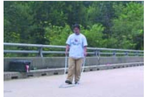
**Figure 2.** Chain drag technique, effective in locating delaminations within several inches of concrete surface, relies on inspector's ability to recognize tone changes.
