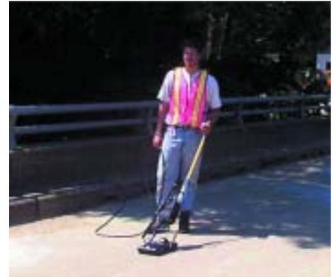
Figure 5. Ground penetrating radar transmits microwave pulses that are reflected from interfaces of materials with different dielectric properties.
