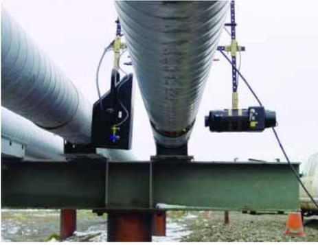
Figure 1. Real-time radiography system set-up to look for corrosion under insulation using a tangential shot. Area of interest for viewing is at the six o'clock position of the pipe.
