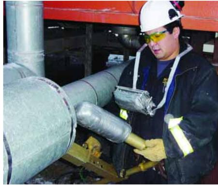
Figure 2. Technician using a lightweight, portable C-arm digital imaging system to look for corrosion under insulation (CUI) on small diameter insulated pipe.
