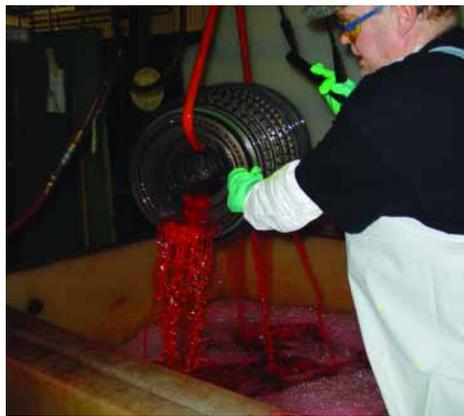
Figure 3. Sling used to transfer component from emulsifier bath to stop bath allows free rotation of part. Rotor can also be turned on drum rotor to allow for free rotation of part.
