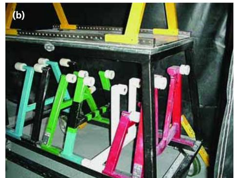
Figure 4. Sets of fixtures conform to varied geometry of parts: (a) fixture used to inspect drum rotor; (b) fixtures loaded on single cart facilitate portability.
