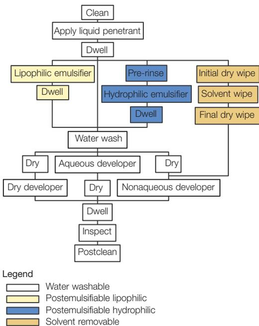
Figure 4. Liquid penetrant processes classified by removal method.
