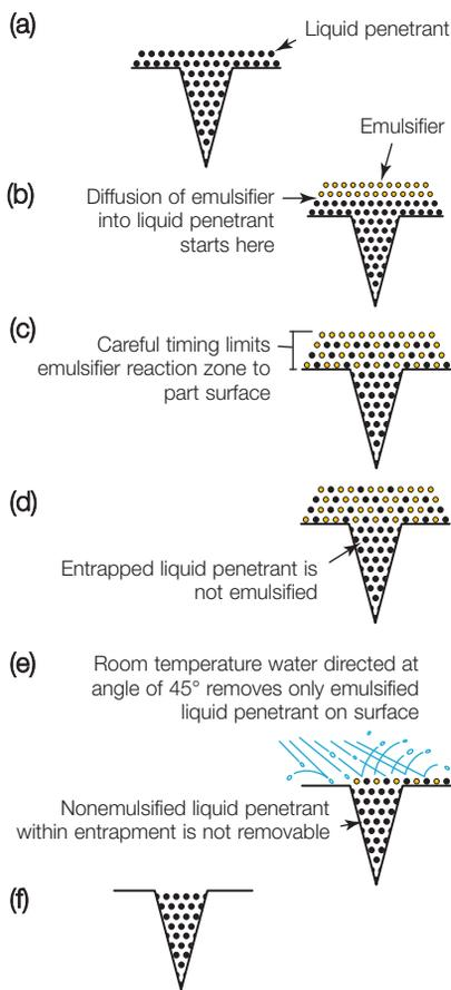
Figure 2. Action of lipophilic emulsifiers: (a) liquid penetration; (b) add emulsifier; (c) solution and diffusion begins; (d) diffusion proceeds; (e) rinsing; (f) clean surface.
