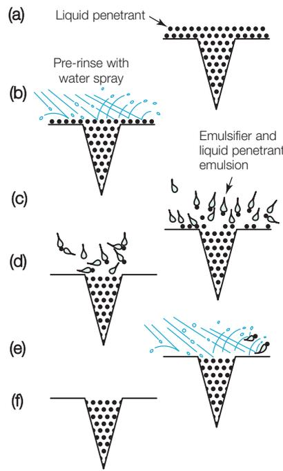
Figure 3. Action of hydrophilic emulsifiers: (a) liquid penetration; (b) prerinsing; (c) detergent scrubbing begins; (d) agitation and emulsification; (e) rinsing; (f) clean surface.
