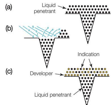
Figure 1. Basic principles of liquid penetrant testing: (a) apply liquid penetrant; (b) remove excess; (c) apply developer.
